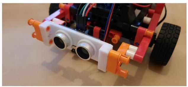
Attach the ultrasonic distance-sensor to the robot.
