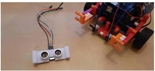
Find an ultrasonic distance-sensor and attach it to the 3D printed module.
