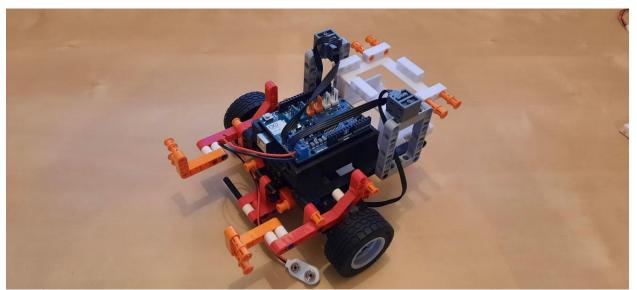
Attach the Arduino R3 Motorshield to the Arduino Uno, and place it on the robot, then connect the cords for the motors and the batteryclip.
