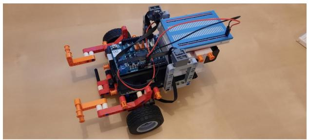
Connect 5V and GND from the Arduino, to the breadboard, using two jumper wires.
