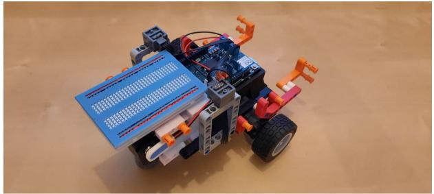
Connect the 3D printed module along with the breadboard, on top of the 3D printed battery holder module, as seen on the image (note that the used breadboard is a prototype, and does not look exactly as a standard breadboard, it works the same however).
