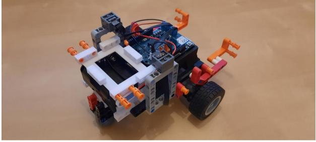
Place the batteryclip inside the robot.
